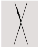
Level 2: Jagged removal along incisions up to 3.2mm on either side.
